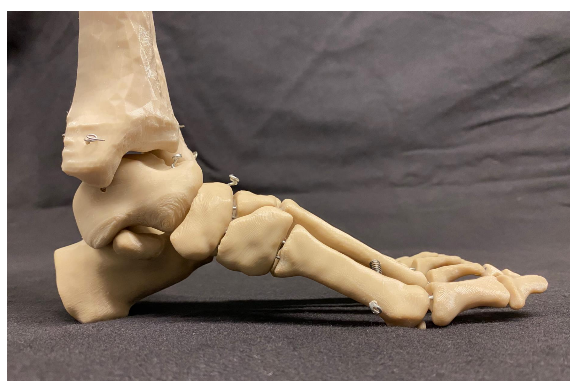
Figure 1: Mechanically post-processed and assembled model of a left foot and ankle. The individual bones are connected by wires and springs to resemble the physiological range of motion of the various joints. The printed model bone of the tibia shows the remnants of the triangular mesh previously used for the 3D model (see Figure 4).
