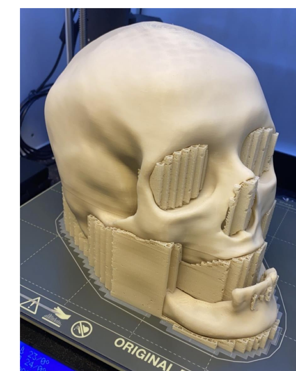
Figure 10: Finished print of a cranium The model with still attached support material is ready to be removed from the print bed and postprocessed by the student.
