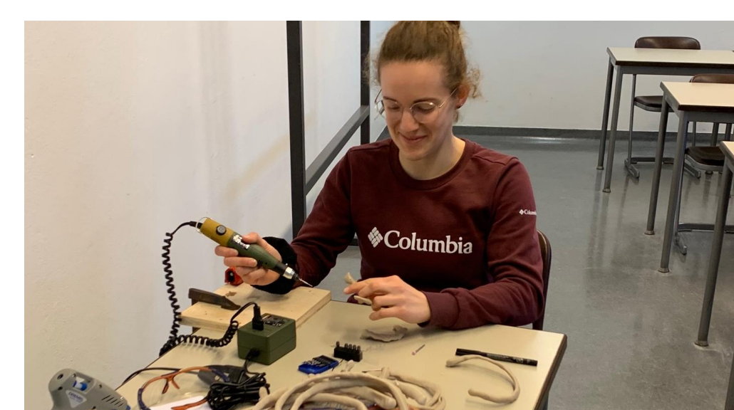
Figure 7: Mechanical postprocessing: In order to remove support structures, improve surface quality and in preparation for assembly of individual joints, students are provided with a variety of necessary materials and tools.
